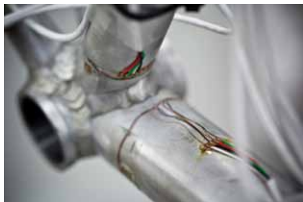
Frame prepared for strain-gauge testing
