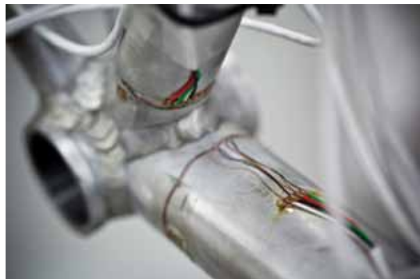
Frame prepared for strain-gauge testing
